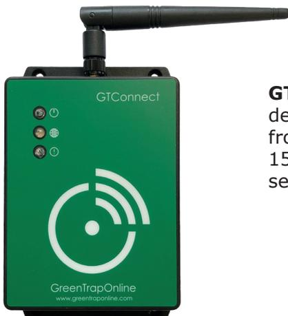
**GTConnect 3.1** - is a specially developed access point that collects data from the GTSensors in a radius of approximate 150-200 meters and sends them to the mail server for processing.
